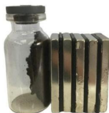
Figure 1. \text{MnFe}_2\text{O}_4 Synthesis results and tests with an external magnet
