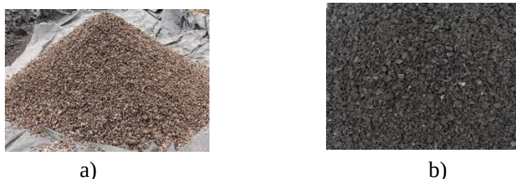
Figure 2. a) cleaned and dried palm shells and b) results of burning palm shells (carbon)
